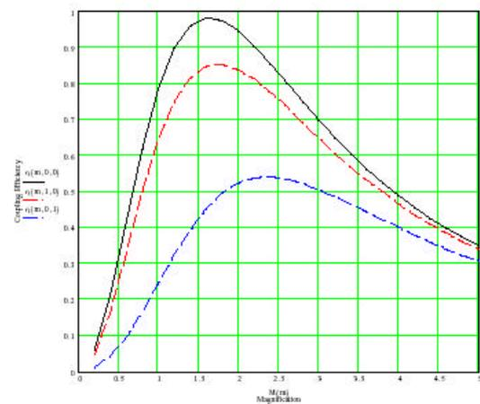
The optical design was evaluated using Code V. This enabled the effects of aberrations to be calculated in estimating the coupling losses - as well as calculating the sensitivities to translation or rotation of the lenses.
