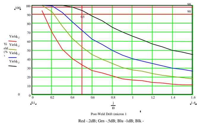
Assuming that the P-WS had a normal distribution, a Monte Carlo algorithm was used to plot the yield as a function of the one-sigma value of the P-WS. *Figure 9* shows how the coupling varies with position vertically. Also shown are the levels corresponding to coupling losses of  $-0.5$ ,  $-1$ ,  $-2$  and  $-3$  dB. The yield corresponding to each coupling level is shown in *figure 10* as a function of the P-WS. If an acceptable loss were  $-0.5$ dB, then the yield for a P-WS of 0.5
