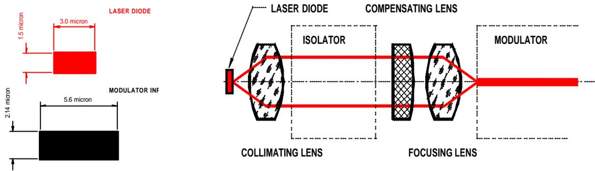
The laser diode output aperture is coupled by the collimator and focusing lenses to the input aperture of the wave-guide modulator. The coupling was calculated using the overlap integral method. The calculation method was extended [1] to include the coupling sensitivity to translation or rotation. This is illustrated by the graph showing how the coupling varies with the linear magnification afforded by the two lenses.
