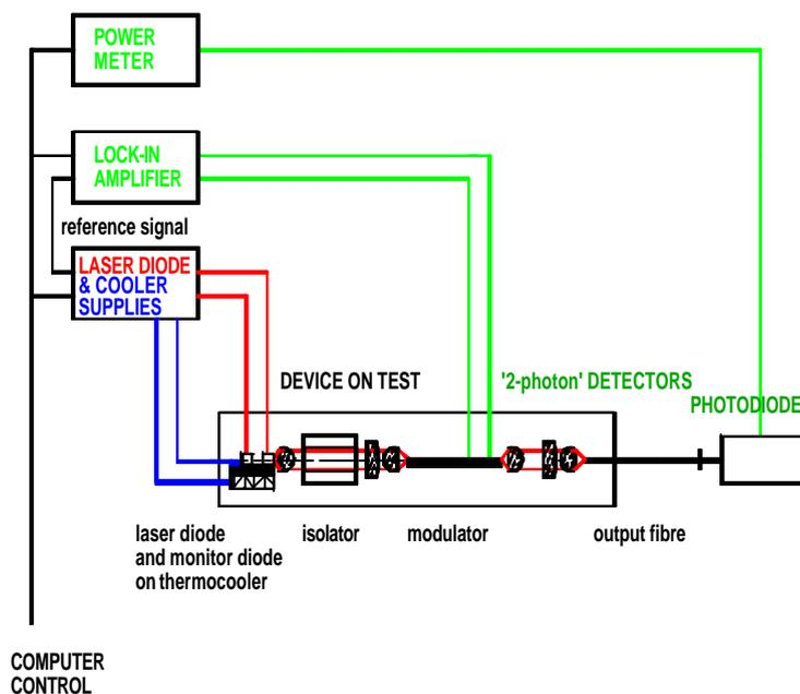
The use of the laser diode modulator and lock-in amplifier lowered the noise floor by almost three orders of magnitude. Combined with the reduced sensitivity to EMI, this increased the volume of space within which a lens could be placed and a signal detected. This produced a significant reduction in the time to 'first light'.
