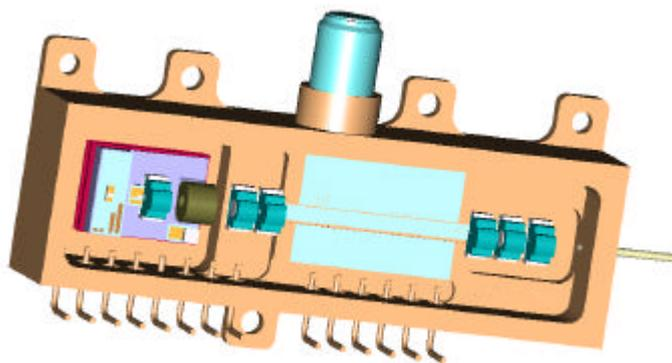
The minimum output power is to be 2mW at 1.53 micron and the modulator is capable of modulation at rates equivalent to 40Gbit/s.
