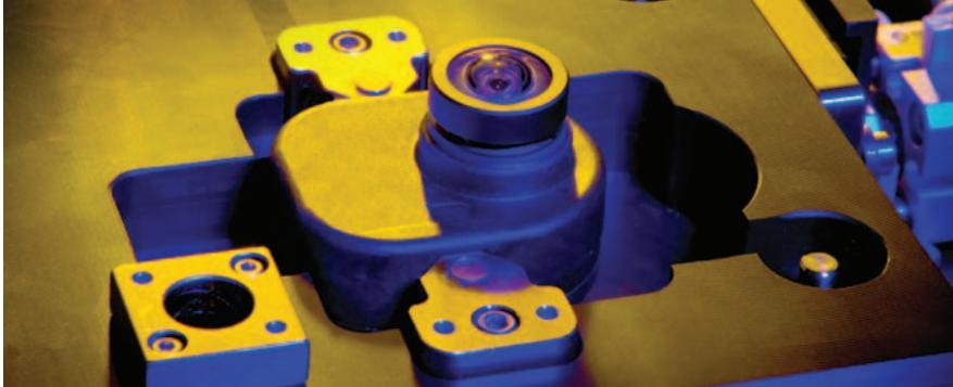
A cell phone camera lens being assembled in a Camera Module Align, Assembly & Test (CMAT) station.
