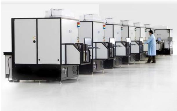
Fig. 8. Example of CMAT Mass Production 5 and 6 DOF Active Alignment Stations
